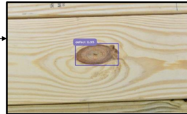
Knot detection, reconstruction [1]; Modeling timber boards with imperfections
