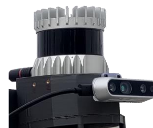
Figure 2: real LiDAR and Camera for data collection.
