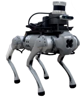
Figure 1: Real Go1 with a mapping system.
