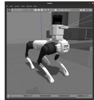
Figure 2: Simulated Go1 with a mapping system in Gazebo.
