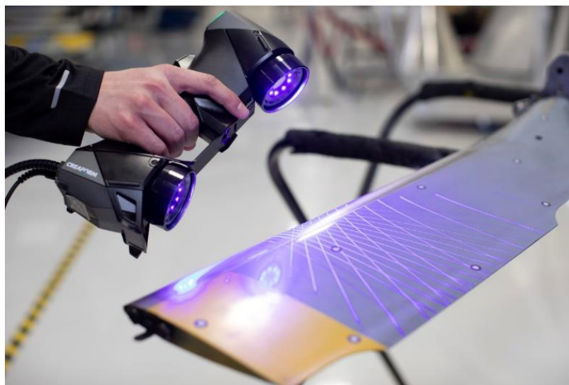
Figure 4 Scanning process with a hand-held scanner
